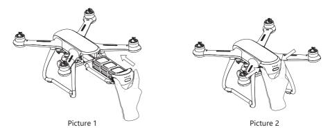
Note: When hearing a "click" sound, the battery is successfully installed in place.
