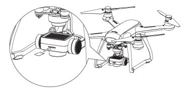
\* Insert micro SD card with the metal side up
